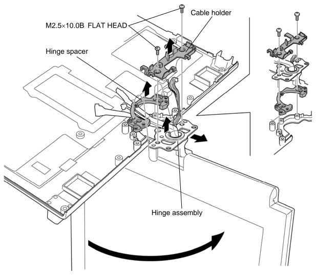
Figure 4-50 Removing the hinge assembly (2)
